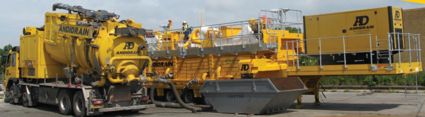
DISAB and Mobile Screening and Dewatering Plant.
