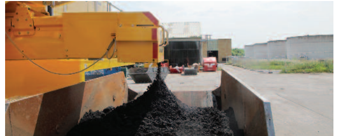
Dry material from Mobile Screening and Dewatering Plant deposited into skip.
