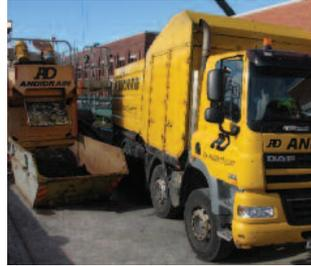
Mobile Screening and Dewatering Plant and JetVac.
